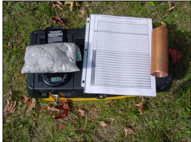
Cellulose core sampling kit
